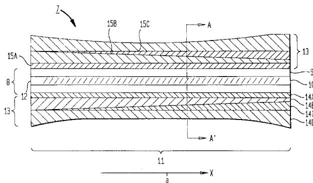
**ARTICLE COMPRISING A TILTED GRATING IN A SINGLE MODE WAVEGUIDE**
