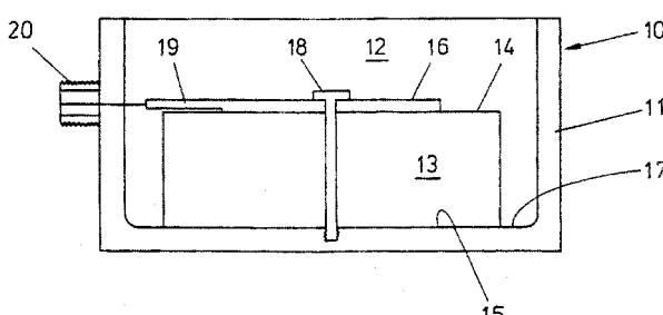
**DIELECTRIC RESONATOR HAVING A FREQUENCY TUNING MEMBER SPIRALLY ENGAGED WITH THE CAVITY**
